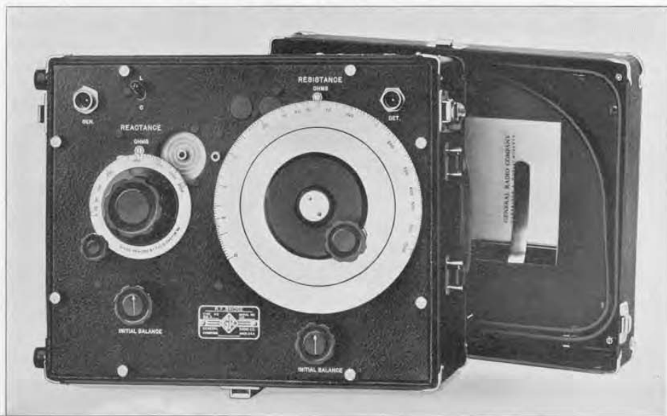
FIGURE 4. Panel view of the bridge. The standard connecting leads supplied with the instrument plug into the jack adjacent to the reactance dial.
